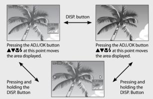
Pressing the ADJ./OK button **34** at this point displays the previous or next image enlarged. When an MP file or a movie is displayed, the display returns to the normal size.
